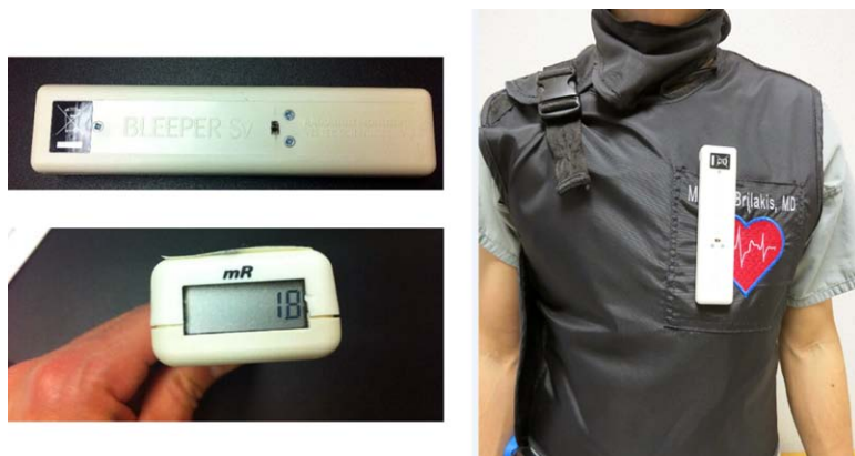
Figure 2. The Bleeper Sv radiation monitoring device (Vertec Scientific Ltd, Berkshire, UK).
