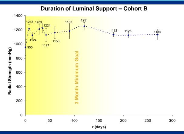
Tests performed by and data on file at Abbott Vascular – in-vitro degradation testing (soaked at 37° C PBS).
